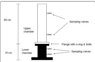
Figure 1 Schematic drawing of the experimental chambers used in the experiments to hydroponically culture eelgrass for DOC exudation measurements. Drawing is not to scale.
