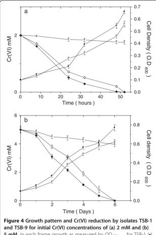
**5 mM.** In each frame growth as measured by  $OD_{600 \text{ nm}}$  for TSB-1 (•) and TSB-9 (o) and chromium reduction by TSB-1 (•), TSB-9 ( $\diamond$ ) and medium alone ( $\Box$ ) have been shown. Error bars indicate standard deviation of triplicate experiments.
